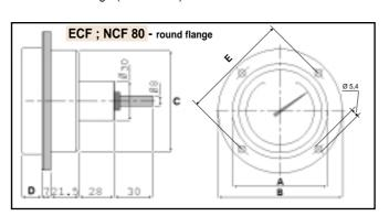
✓ ESF 80 ✓ ECF 80 Scale's end can be reached with a speed of between 200 and 3000 turns/minute. • Materials: body in Nylon PA66 loaded glass - flange (in mod. ECF) in ABS.
