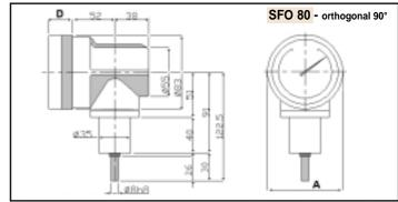
Scale's end can be reached with speed of between 200 and 3000 turns/minute. • Materials: body in Nylon PA 66 loaded glass - flange in ABS.
