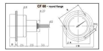
✓ SF 60 Scale's end can be reached with speed of between 100 and 5000 turns/minute. ❖ Materials : body in aluminium flange (in mod. CF) in aluminium.
