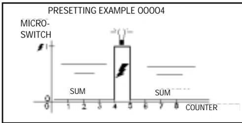
Δ **C** - 5-digit presetting; upon reaching the preset value, a micro-switch is activated for a **single unit duration**
