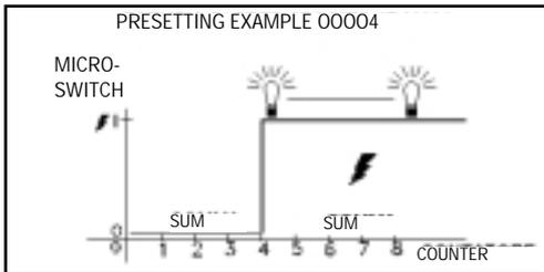
Δ **E** - 5-digit presetting; upon reaching the preset value, a **permanent micro-switch** is activated. When resetting the device, the micro-switch returns to its initial position
