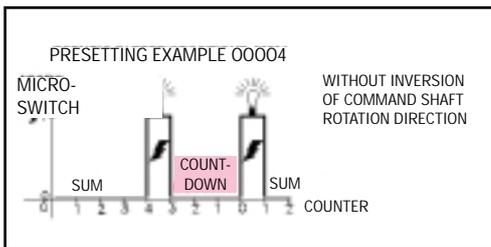
Δ **PVC** - 5-digit preset = PERIODICAL VARIABLE. After presetting a chosen value (period), the totalizator adds on until reaching the preset value, then, **without inverting the rotation direction of the command shaft**, it counts down until zero, then adds on again, etc... Both when the preset value (variable) is reached and at the moment of the formation of 0000 (fixed), the device activates a micro-switch for the whole duration of a **unit**.
