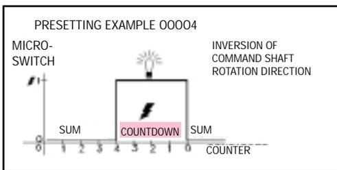
Δ **F** - 5-digit presetting; similar to Model ΔE. When release occurs once the preset value is reached, the micro-switch remains excited until reaching the ZERO value by inverting the command shaft rotation direction. It is therefore possible to use two different circuits: one during the active phase (SUM) and the other during the negative phase (COUNTDOWN) after reaching a preset value.
